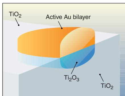
**Gold that works:** Proposed structure of active gold nanoparticles in which reduced TiO<sub>2</sub> accumulates under gold islands, as first shown in (19).
